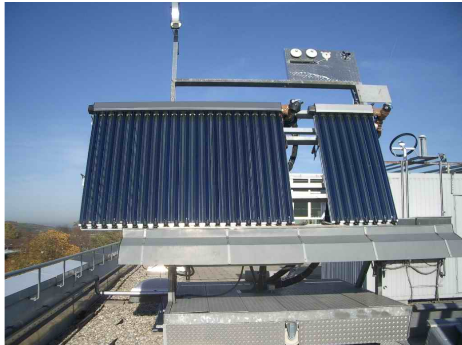
Figure 1: Picture of the collector VacoSol CPC 21 mounted on the test facility of Fraunhofer ISE
